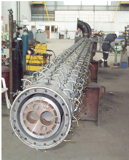
Dual-fuel burner of calciner cyclone Exchanger. Dry method of cement production. Coal dust / liquid or gaseous fuel. Power 40 MW
